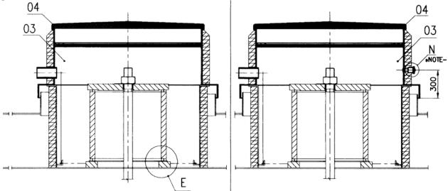
• Install collecting electrode suspension frame supplied against Clause No. 1A/1.1 and weld the same as per standard ESP erection procedure.
